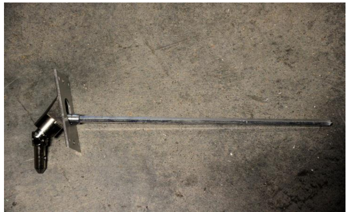
11. Cut through wall rod to length needed. It can go all the way through the gearbox. Put crank rod through wall into gearbox.
