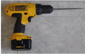
Power driver with 6" Phillips #2 tip is best tool to install the shutter.
